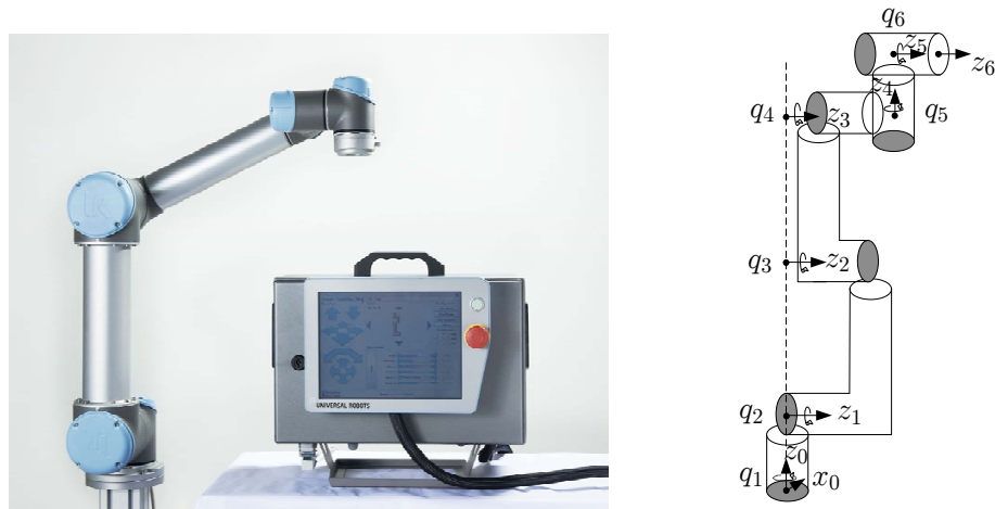
Fig. 2. UR5 robot and its joint coordinate system. Left: UR5 robot and PolyScope GUI [15]; Right: joint coordinate system.
