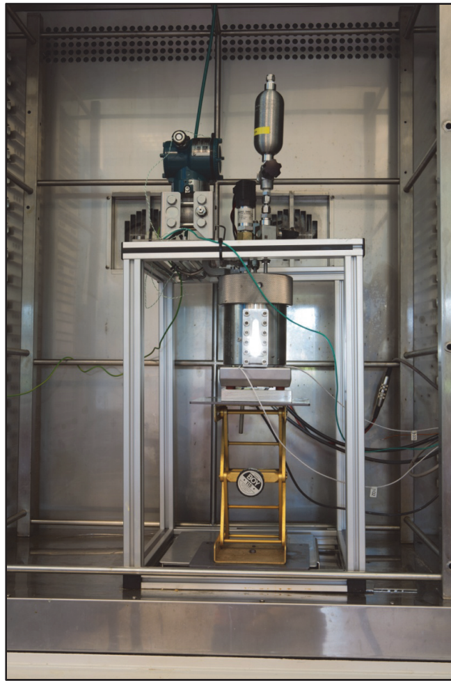
Figure 7.2 Image of the high-pressure equilibrium cell together with the gas cylinder, pressure sensors and other parts, inside the temperature chamber.
