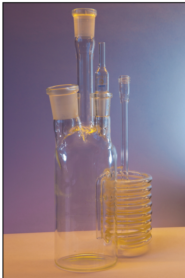
Figure 4.7: Image of the cell shown in Figure 4.1. The gas inlet is a vertical glass tube.
