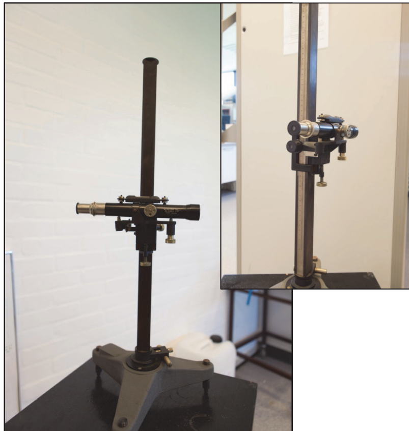
Figure 7.3: Image of the cathetometer used to determine the liquid volume inside the equilibrium cell.
