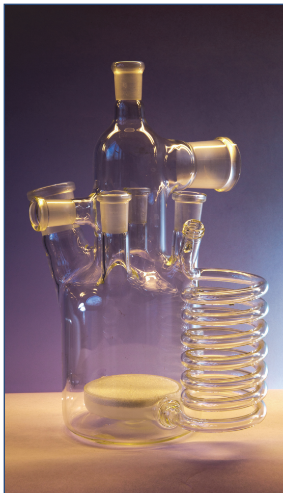
Figure 4.8: Image of a second equilibrium cell fabricated during this work. The gas inlet is a glass sieve.
