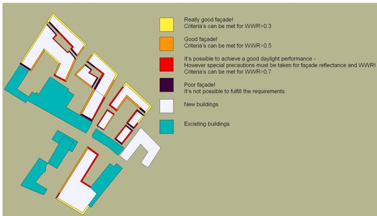
Figure 6.3: An application example of the results, for planning of a new urban area. Note: The color mapping shown here corresponds to the daylight performance for the ground level.
