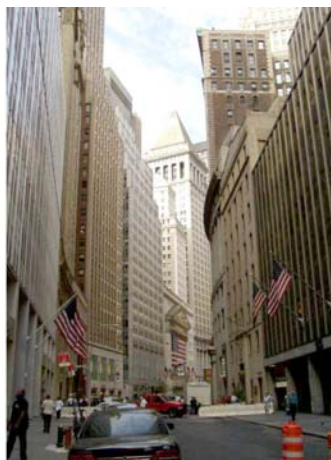
Figure 2: Wall Street Canyon. Façade reflectance approximately equal to 45% - 55%.
