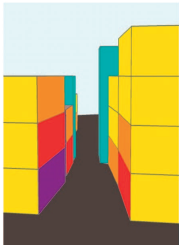
Fig. 9. An application example of the EvUrbanplan tool for designing the urban fabric. Note: The street width is 10 m, each floor has a height of 5 m and the colour mapping follows the coding in Table 1 and Figure 8.
