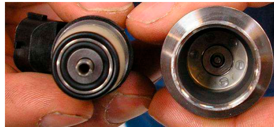
Figure 3 - Photo of disassembled injector showing O-rings
