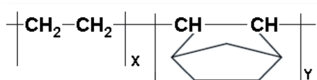
Figure 1: chemical structure of TOPAS, consisting of ethylene and norbornene subunits. [adapted from TOPAS Advanced Polymers]
