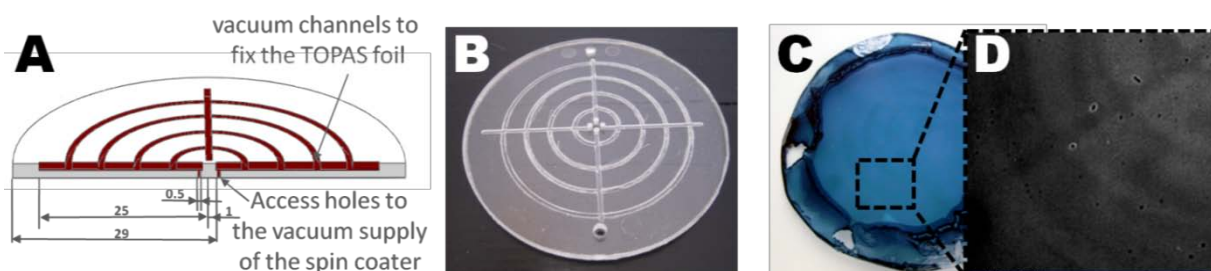
Figure 66: A) Sketch of the fabricated chuck with four straight and four circular vacuum channels (red) to attach the TOPAS foil during spin coating, B) Photograph of the fabricated spin coating chuck, C) coated TOPAS foil with polymerized PEDOT film, and D) magnification of a part of the polymerized PEDOT layer. The magnification is presented in grayscale for a better visualization of the chuck marks (bright areas).
