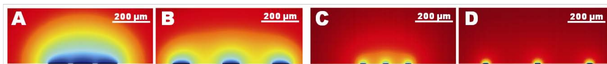
Figure 60: Finite element modelling of the redox active species concentration for \text{Ø}100 \text{ }\mu\text{m} (A + B) as well as \text{Ø}30 \text{ }\mu\text{m} (C + D) electrode arrays with 130 \text{ }\mu\text{m} (A + C) and 300 \text{ }\mu\text{m} (B + D) center-to-center spacings, after running amperometric measurements for 90 \text{ s} . The graphs are presented as cross-sectional views through the three center electrodes of each array (dark red: initial concentration; black: zero concentration).
