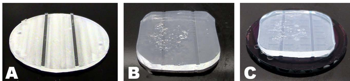
Figure 88: Process of PEDOT deactivation by incubation with aqueous sodium hypochlorite using agarose stamping. A) After a mold fabrication, B) the mold surface was replicated in an agarose gel. C) The gel was loaded with aqueous sodium hypochlorite and pressed for 5 min against the structured PEDOT/TOPAS wafer. Deactivation took place only at contact areas, PEDOT at embossed areas as well as at the two lines of the mold structure remained conductive.
