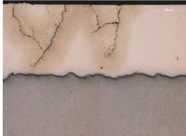
Figure 21: Cross-section of Crack
