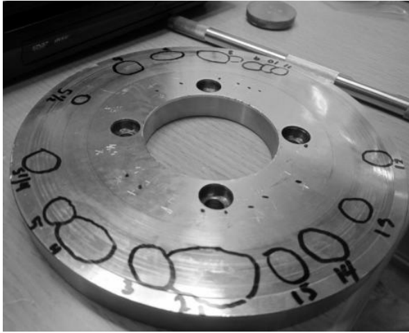
Figure 17 : Disc With Fatigue Damages
