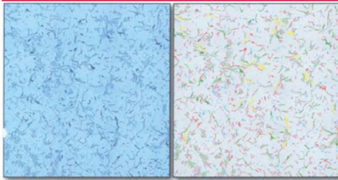
Fig. 1. Left: Unetched micrograph. Right: Graphite detection. Detection area is totally 83mm 2 .
