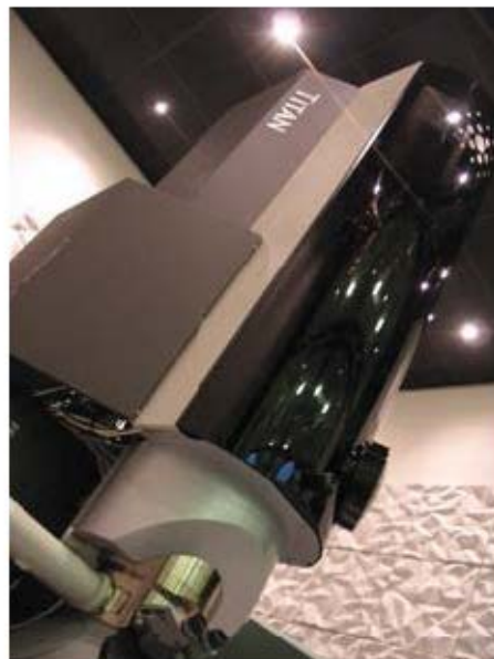
Investigations performed using FEI TITAN 300KV analytical TEM with High Angle Annular Dark Field (HAADF)
