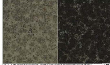
Fig. 1 Left: etched micrograph. Right: Deep etched micrograph (Hard phase)
