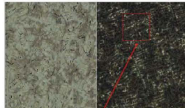
Fig. 1 Left: etched micrograph. Right: Deep etched micrograph (Hard phase)
