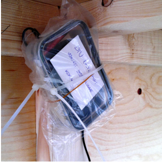
Figure 3. Nokia N900 Bluetooth scanner in a protective box attached under a beer booth counter.
