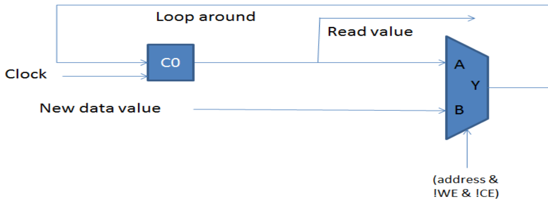
Figure 13 General structure of a memory array
