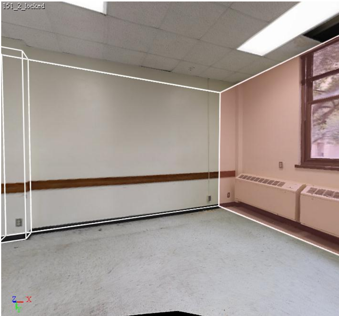
Figure 32 Geometry model does not fit to texture of panorama
