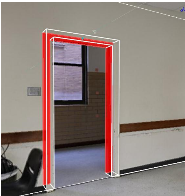
Figure 23 Extrude face for door frame
