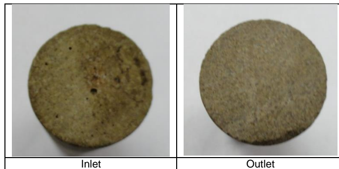
Fig. IV.7– Inlet and outlet for a core tested with 5 wt% HCl, 10,000 ppm \text{Fe}^{3+} , GLDA:Fe = 2:1.
