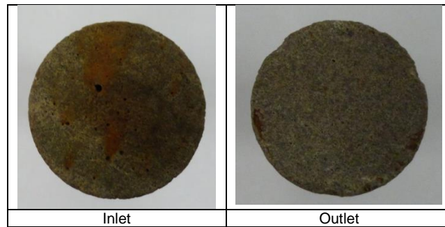
Fig. IV.6– Inlet and outlet for a core tested with 5 wt% HCl, 10,000 ppm \text{Fe}^{3+} , GLDA:Fe = 1:1.
