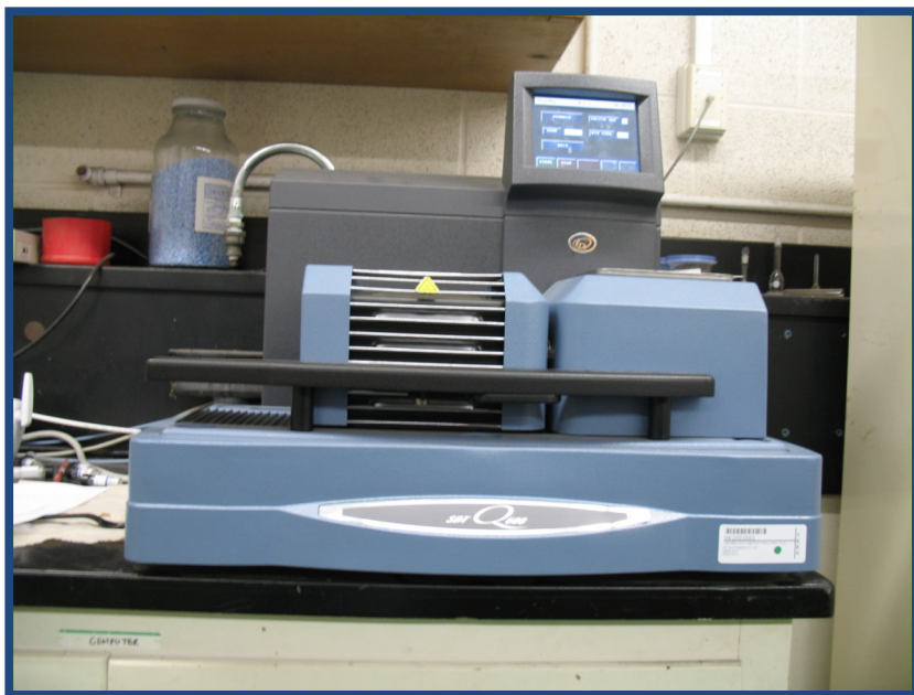
Fig.3-5. TA Instrument SDT-Q600 DSC-TGA.
