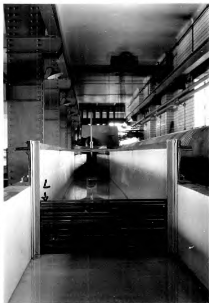
PHOTOGRAPH SHOWING REGULATION WEIR L. THE VENTURI FLUME MODEL & POINT GAUGE ARE SHOWN UP STREAM.
