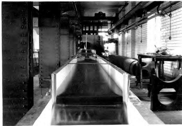
PHOTOGRAPH SHOWING WATER FLOWING D.S OF MODEL & OVER THE REGULATION WEIR L , LOOKING U.STREAM
