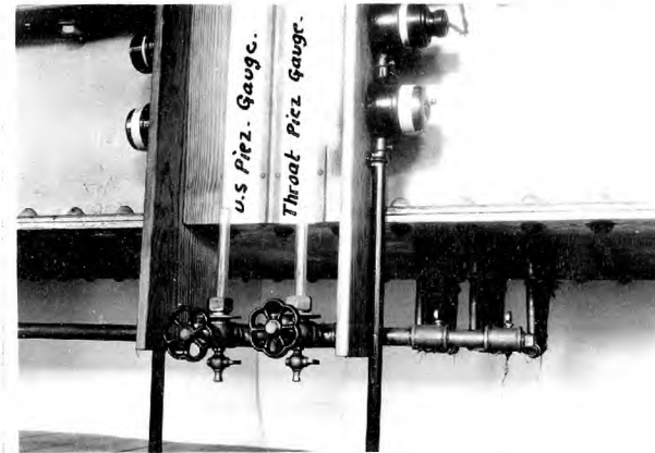
PHOTOGRAPH SHOWING PIPE CONNECTIONS BETWEEN THROAT PRESSURE HOLES & THROAT PIEZOMETER GAUGE .
