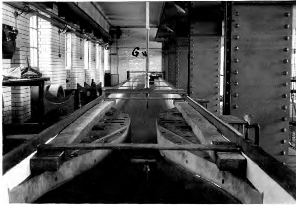
PHOTOGRAPH SHOWING WATER FLOWING THROUGH VENTURI FLUME MODEL I , LOOKING DOWN STREAM. THE BOTTOM OF THE DROPPING WATER SURFACE CURVE IS SHOWN AT THE REFLECTION OF THE POINT GAUGE G
