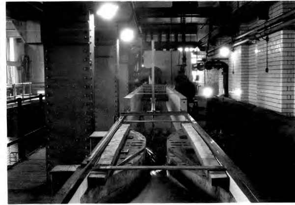
PHOTOGRAPH SHOWING WATER FLOWING THROUGH VENTURI FLUME MODEL I , LOOKING UP STREAM . THE DROP INSIDE THE THROAT IS MARKED BY THE LIGHT REFLECTIONS.
