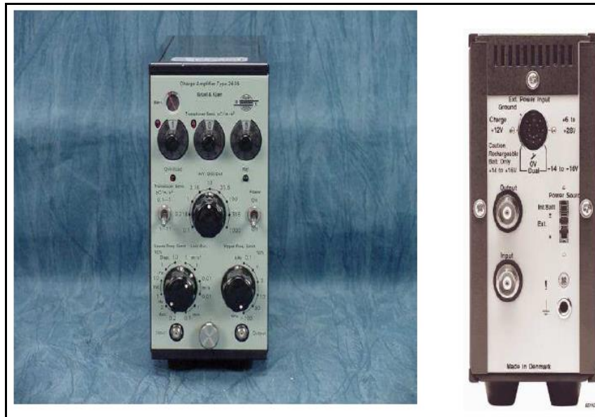
Figure 6.8 Face of B&K charge amplifier type 2635 (left), back (right) [278].
