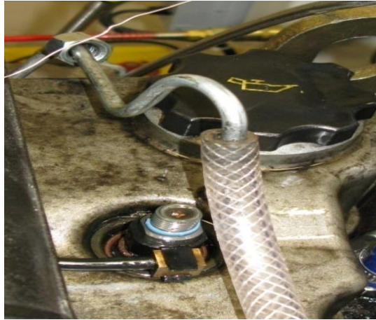
Figure 6.19 Arrangement for total misfire.
