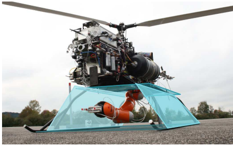
Fig. 9. Helicopter/ Manipulator system with illustrated virtual walls, to avoid self-collision.
