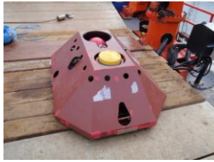
Fig. 5 ADCP used at SWMTF in its frame
