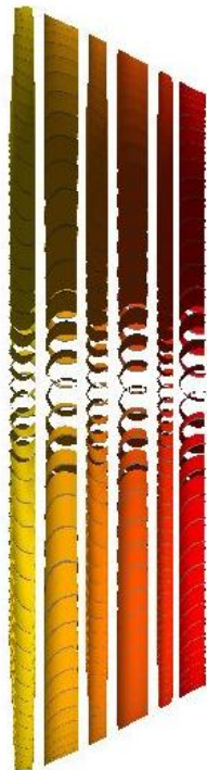
Figure 6.10 - T-AXI three-spool IPT blading, side view
