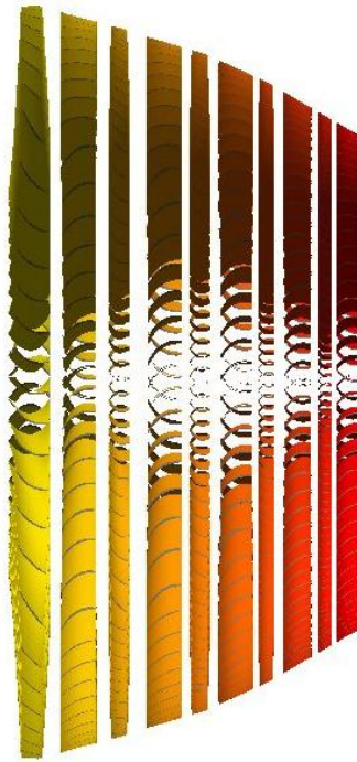
Figure 6.3 - T-AXI two-spool LPT blading, side view
