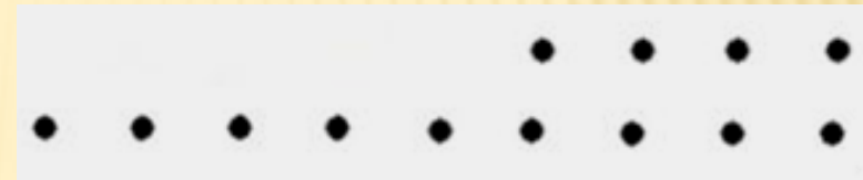
Warp arrangement for 'T' formation in the folded manner
