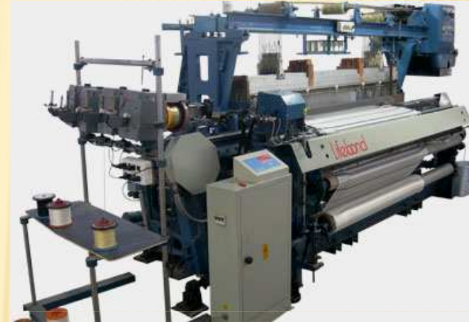
Dobby loom for small designs (saree weaving, silk dhotis with borders)
