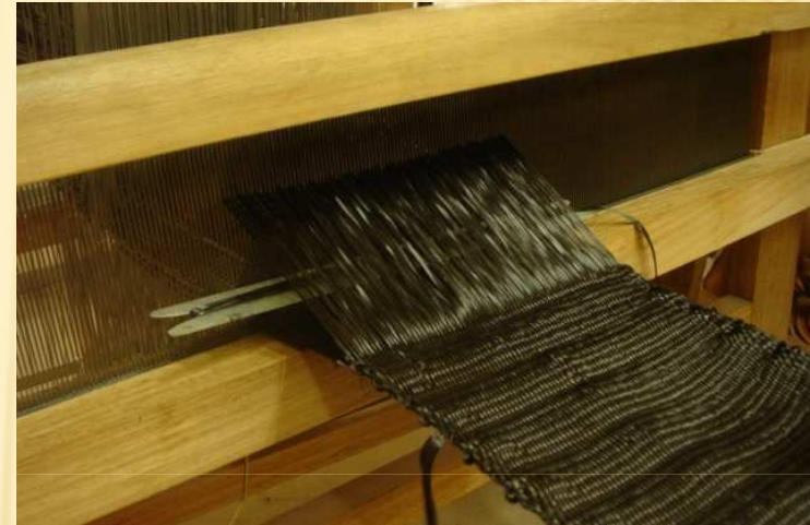
Weft Insertion through the shed
