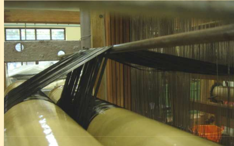
Warp passing over back rest
