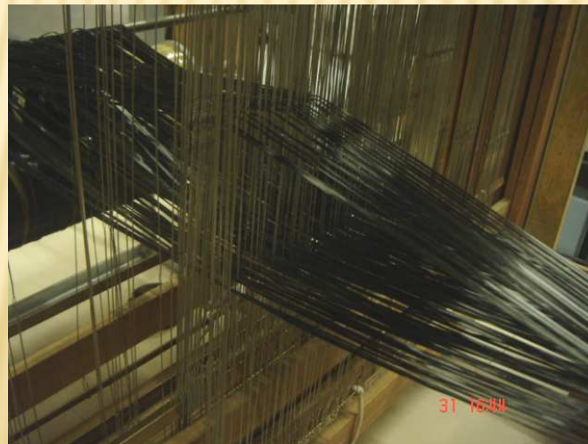
Warp passing through heald wires
