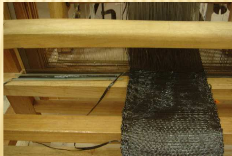
Pushing the inserted weft to the cloth fell
