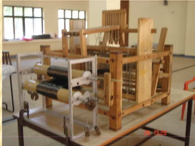
Multiple beam preparation
