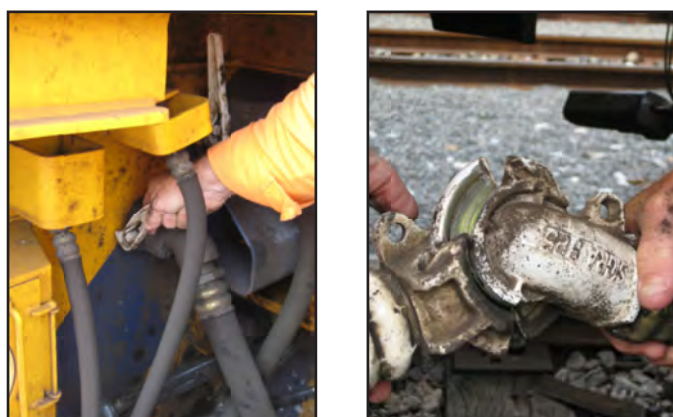
Figures 3A & B: Coupling and Uncoupling brake hoses
