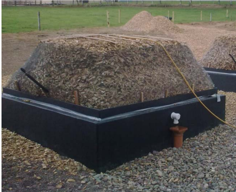
Figure 1.2 A woodchip biofilter in operation (Carney et al., 2011).
