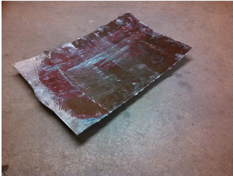
Figure 3 - A sheet metal approximation of a paraboloid, with aluminum coated mylar.
