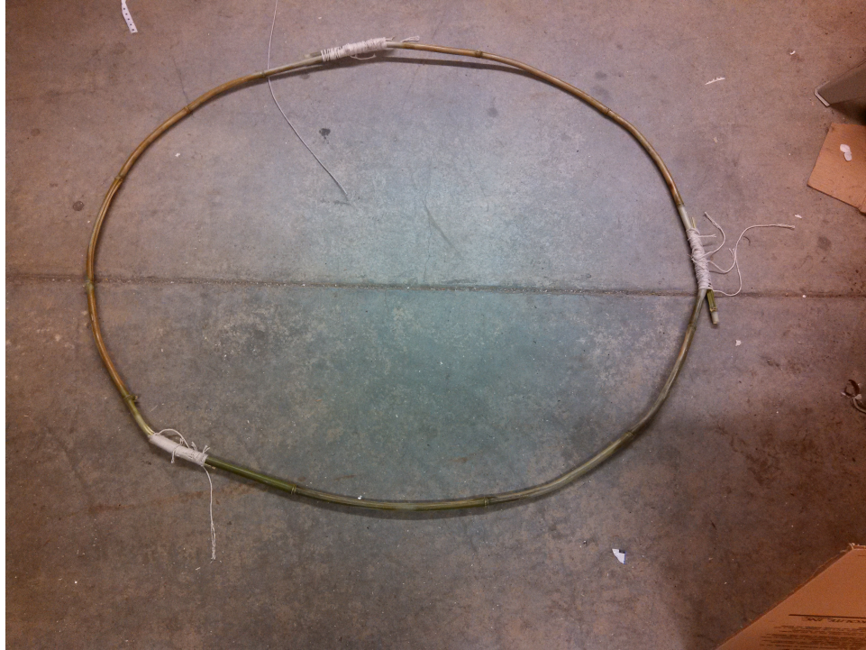
Figure 5 - Hoop approximately 3 feet in diameter, bent with a blowtorch and twine.
