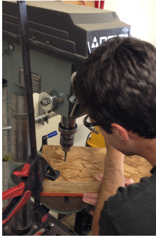
Figure 10 - Jason drilling pilot holes for the alignment thread rod.
