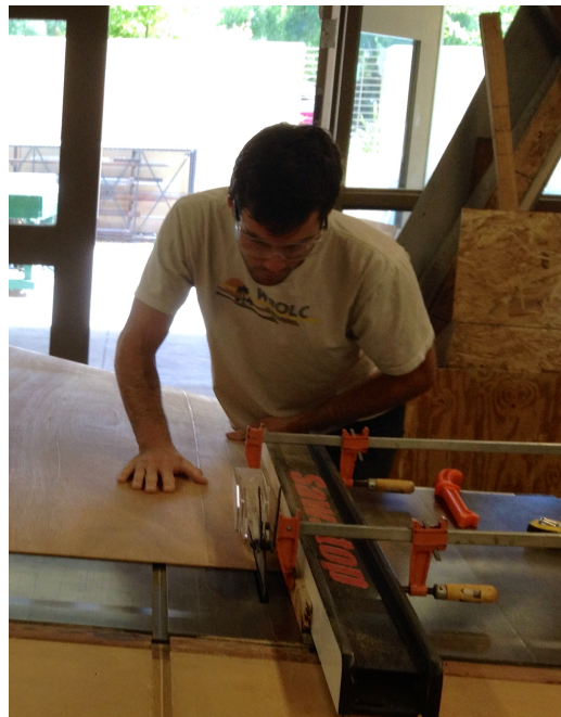
Figure 9 - Jason using a table saw to cut support slats for the Scheffler dish.
