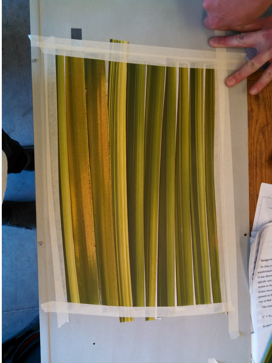
Figure 6 - Initial layout of plant leaves to make a composite lattice.
