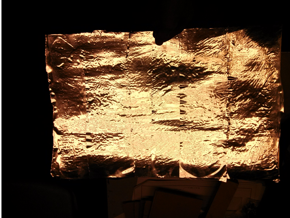
Figure 4 - Picture of sheet metal approximation. The photograph was taken close to the focal point of the dish. All the illuminated portions of the sheet are successfully focusing light, whereas the dark areas are not.
