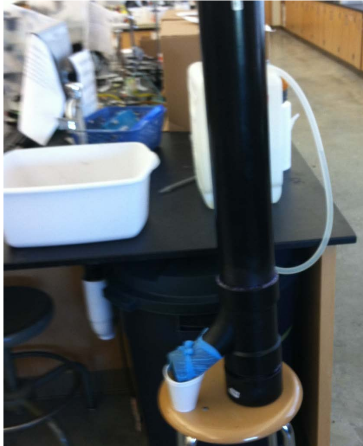
Figure 14: The Single Pass Peat Filter Ready for Testing
