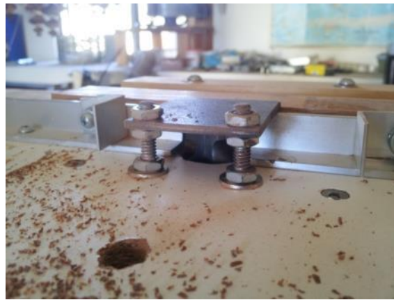
Figure 1.3. Steel plate used as current cutter head safety guard.
