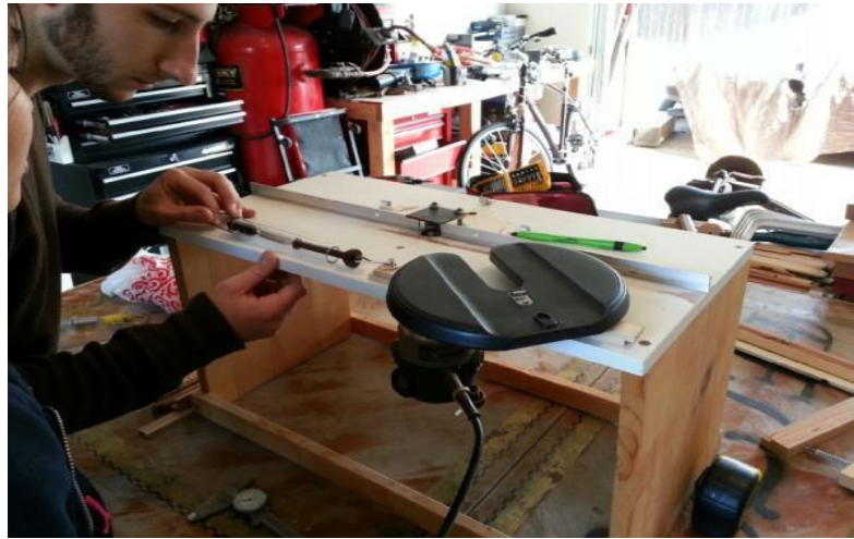
Figure 3.9. Testing to determine coefficient of friction between redwood and the router table surface.
