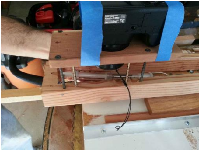
Figure 3.10. Apparatus used to record force needed to push slats.
