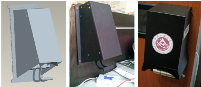
Figure 2-11 Schematic and picture of the image acquisition device
