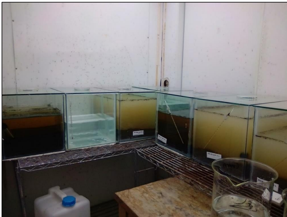
Plate 3.5 Partial experiment setup within the environmental chamber showing the tanks with different surface area to volume ratios and the two sediment types after inundation.
