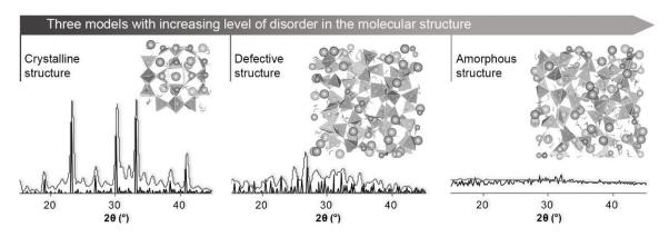
Figure 1 – Three different geopolymers molecular models with increasing level of disorder but with comparable Si:AI. The level of disorder is characterized by the corresponding X-ray diffractions.
