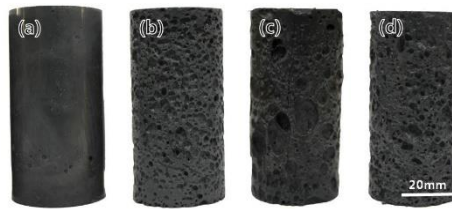
Figure 1 – Solid (a) and cellular structured fly ash-geopolymer cylinders ((b)-(d)). Aluminum concentration is 0.025 wt% (b), 0.05 wt% (c) and 0.10 wt% (d).
