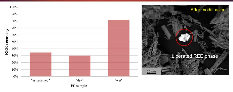
Wet/hydrothermal way of PG modification =>
