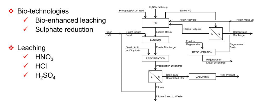
Resin-in-Leach process developed and piloted at Mintek (2011-2012):
