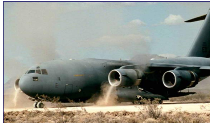
Aircraft Engines Ingesting Sand on Runway
