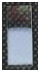
Figure 1 Photograph of electrophoreticallydeposited titania-nanosheets film onto ITOcoated glass substrate (anode). The deposit area was 13 mm x 8 mm.
