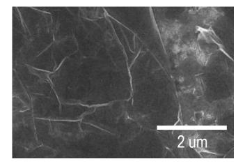
Figure 2 SEM image of electrophoretically-deposited titaniananosheets film onto ITO-coated glass substrate.
