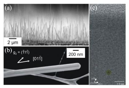
Figure 1 – SEM and TEM micrographs of Cu nanowhiskers
