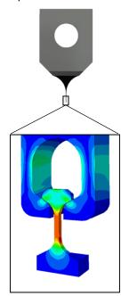
Figure 1 – Silicon gripper (top) and dumbbell bone sample (bottom)
