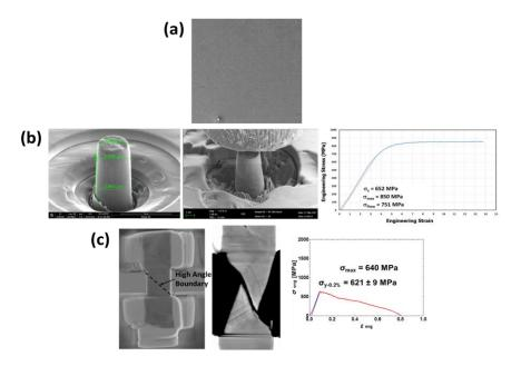
Figure: Small-scale mechanical testing at CNL: (a) Nanoindentation testing for spatial mapping, (b) Microcompression tests for bulk material property evaluation, (c) Micro-tensile testing of specimens with isolated micro-structural features
