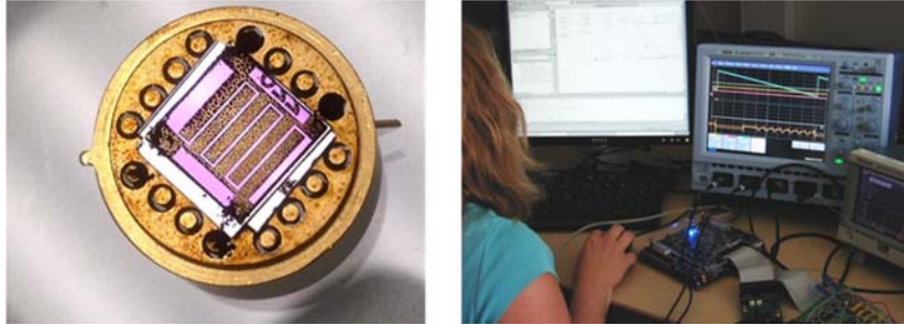
Figure 9. (left) Super-capacity for energy harvesting device integrated in connected objects ( After Toulouse center activity report. ) and (right) Embedded electronics for connected objects ( After Grenoble center activity report. ). These devices and circuits are fabricated and designed by the students on the CNFM platforms.
