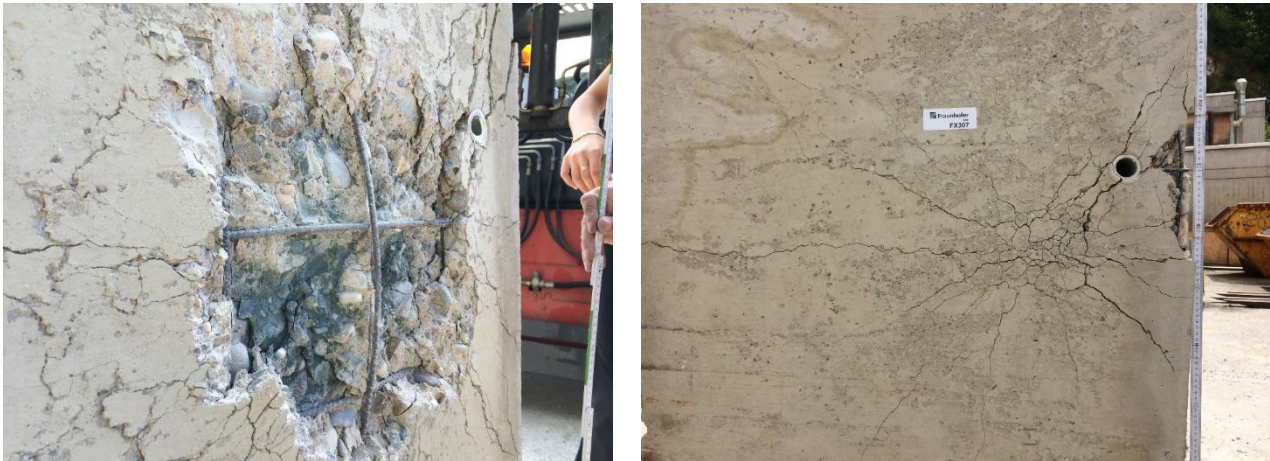
Figure 1: Backside of a concrete slab exposed to explosive impact without (left) and with (right) an 8 cm cover of the developed concrete mixture (by courtesy of Fraunhofer EMI)
