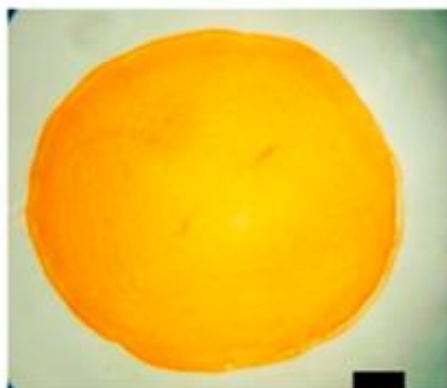
Figure 1 –Patterns formed upon evaporation of drops containing ellipsoids: coffee-stains (top) and uniform deposit (bottom). The scale bar is 0.5 mm
