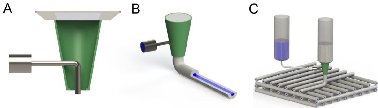
Figure 1: Principle of core/shell plotting. (A) Double extrusion nozzle, (B) Core/shell extrusion, (C) 3D Plotting of a core/shell scaffold
