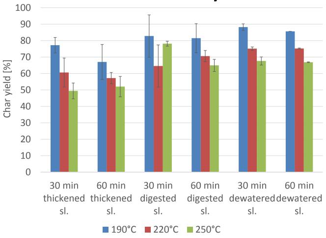
HTC allows sludge reduction: yield of Chars was 49-88% in function of temperature, residence time and kind of sludge.
