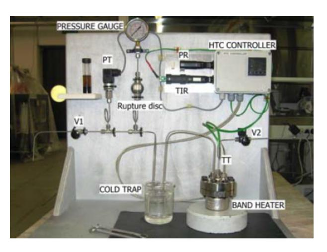
Stainless steel lab batch reactor (50mL) capable to withstand high pressure (140 bar) and temperature (300 °C) was used. Temperature and pressure were measured with a Thermocouple and a pressure transmitter, respectively. A copper gasket was used to ensure perfect sealing
