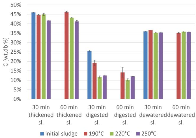
Carbon content increases only in two cases. This is due to high ash content and mass reduction caused by the degradation of the organic fraction during the HTC process.
