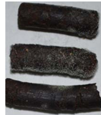
Pellets made from torrefied canola straw with 5% binder
