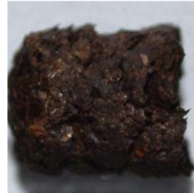
Torrefied canola pellets with 5% binder after immersed in water and drying
