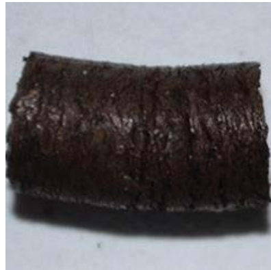
Torrefied canola pellets with no binder after immersed in water and drying
