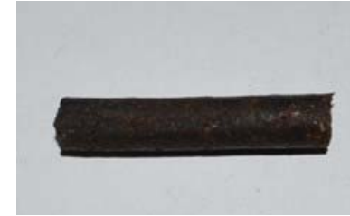
Pellets made from torrefied canola straw with 5% binder
