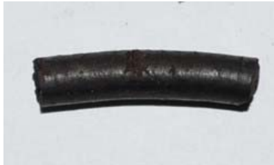
Pellets made from torrefied canola straw no binder
