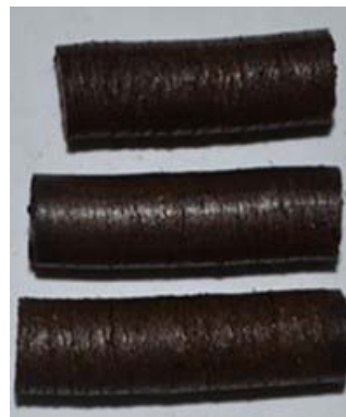
Pellets made from torrefied canola straw no binder
