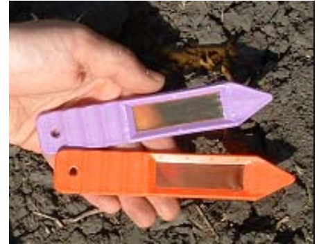
PRS ion-exchange probes used to assess availability of major soil nutrients
