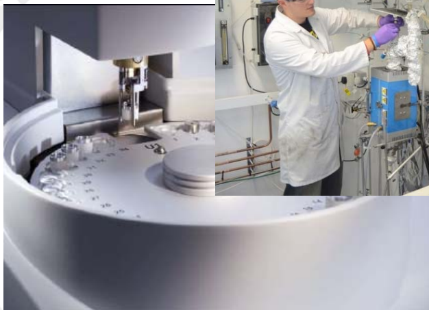
Automated TGA/DSC instrument for biomass pyrolysis and biochar characterisation, capacity up to 5g .
