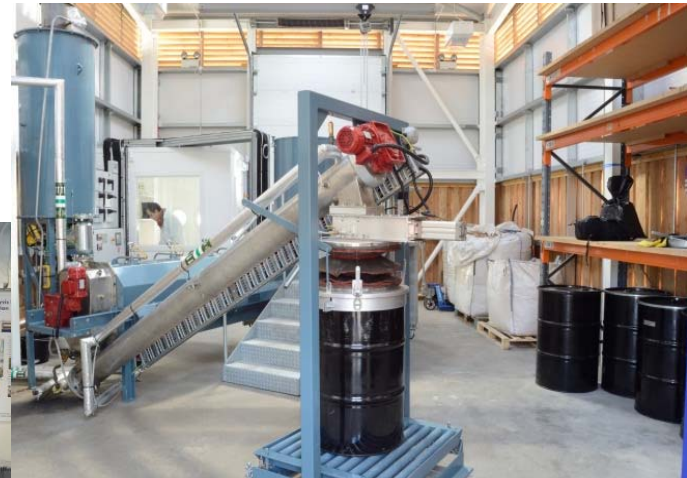
Pilot-scale continuous pyrolysis unit with capacity of up to 50 kg/h of biomass, mean residence time 5-60 min., and temperature range up to 850 °.
