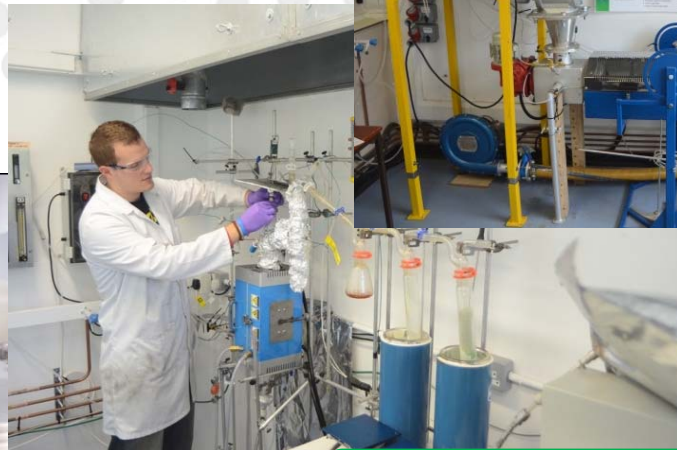
Bench-scale batch pyrolysis with capacity of up to 100g , operating temperature range up to 1100 °C and heating rate from <math><1^{\circ}\text{C}/\text{min}</math> to <math>>100^{\circ}\text{C}/\text{s}</math>.
