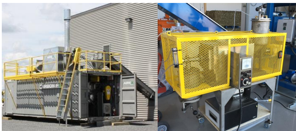
Figure 1 – Right side: the pilot-scale industrial torrefaction unit at CTRI (CarbonFX, Airex Energy); Left side: the prototype furnace developed at CTRI for activation.
