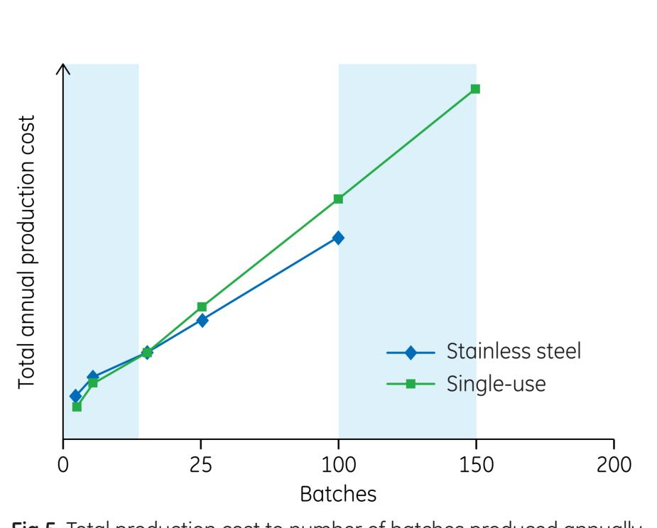
Fig 5. Total production cost to number of batches produced annually in single-use and stainless steel facilities.
