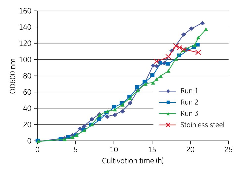
Fig 1. Cell growth in XDR-500 MO at studied feed rates. Cell growth even at lowest feed rate was comparable with stainless steel bioreactor.
