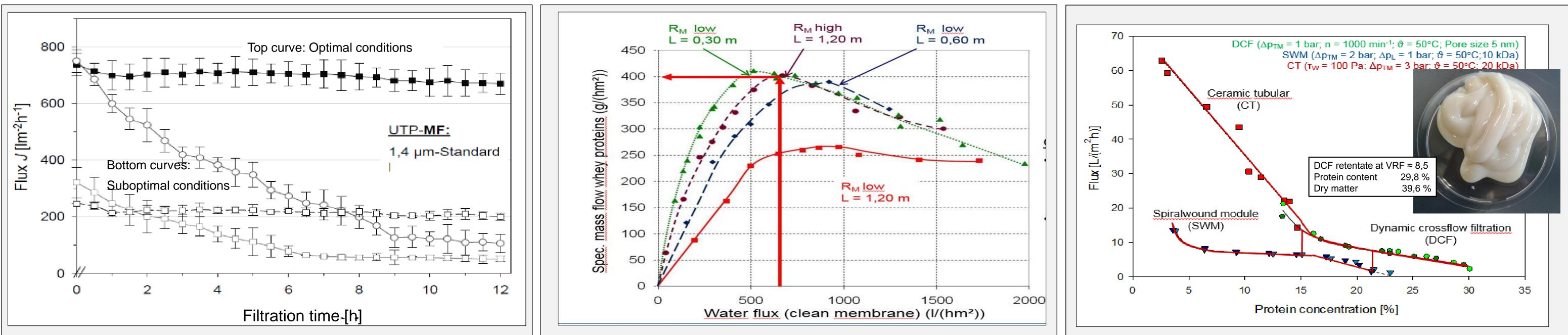
UTP mode reduces deposit formation and stabilizes flux
