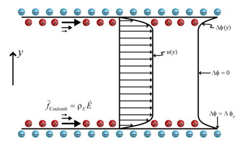
Electroosmosis is a preferred liquid-delivery tool in microfluidics because it is much more efficient at micro-scale than pressure-driven flows.
