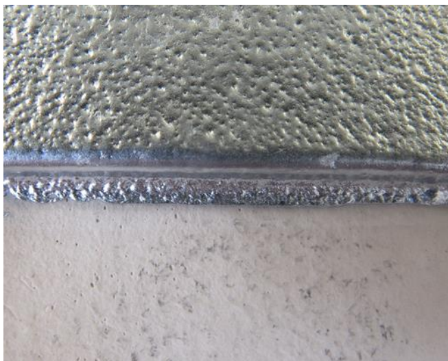
Figure 2 – Contact area of solidified aluminum and syntactic foam core (low pressure die casting).
