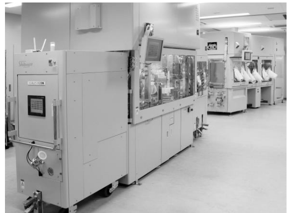
Fig. 2 Cell manufacturing system based on fMP
