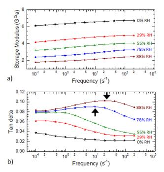
Figure 1 –Nanoindentation-based mechanical spectroscopy of S2 secondary wood cell wall layers in latewood loblolly pine. a) Storage modulus and b) tan delta as a function of frequency and humidity.
