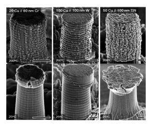
Figure 1 – High resolution SEM images of micropillars micro-machined within the nanolayered layered films and compressed in situ SEM at 25°C and 200°C. Length of micron-marker is 500 nm.
